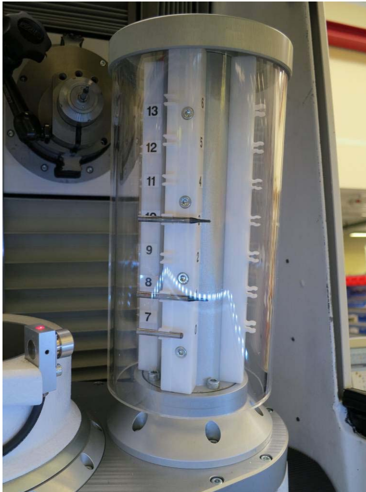
Picture 23. Tool changer with tools
